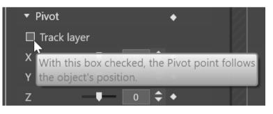
check the Track layer box the pivot point values become relative to Position values and therefore the Pivot Point follows the layer as it moves across the video frame so that you don't need to keyframe it separately
